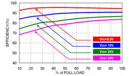
**43PSR1.0-5P0 Efficiency vs. Output**
