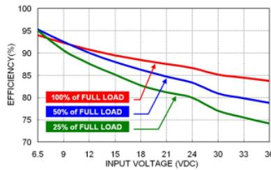
**43PSR1.0-5P0 Efficiency vs. Input**
